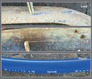
Most residential water service lines in Concord are made of lead, copper, or plastic. Lead service lines are generally a dull gray color and are very soft. You can identify them easily by carefully scratching the service material with a key. If the pipe is made of lead, the area you've scratched will turn a bright silver color.
